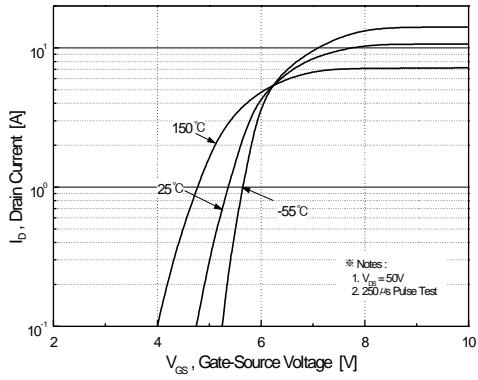
**Figure 2. Transfer Characteristics**
