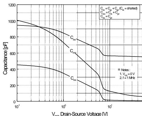
**Figure 5. Capacitance Characteristics**
