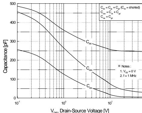
**Figure 5. Capacitance Characteristics**
