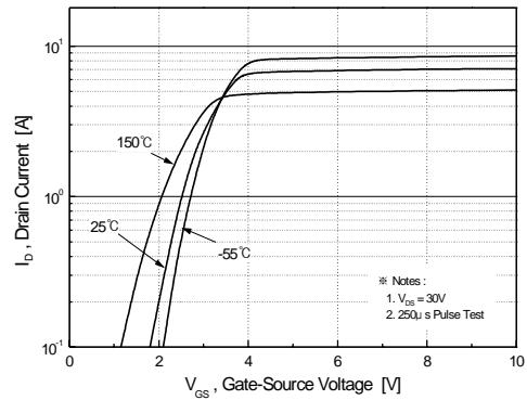
**Figure 2. Transfer Characteristics**
