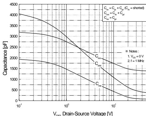
**Figure 5. Capacitance Characteristics**
