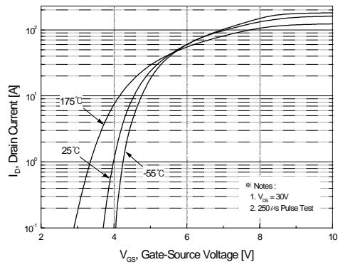
**Figure 2. Transfer Characteristics**
