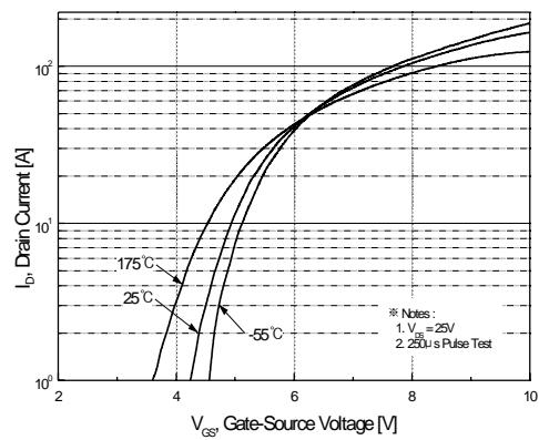
**Figure 2. Transfer Characteristics**
