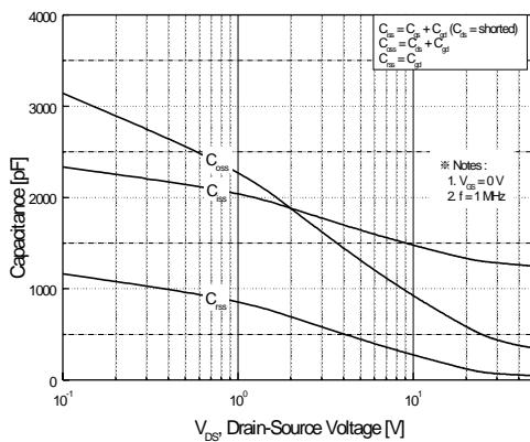
**Figure 5. Capacitance Characteristics**
