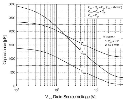
**Figure 5. Capacitance Characteristics**
