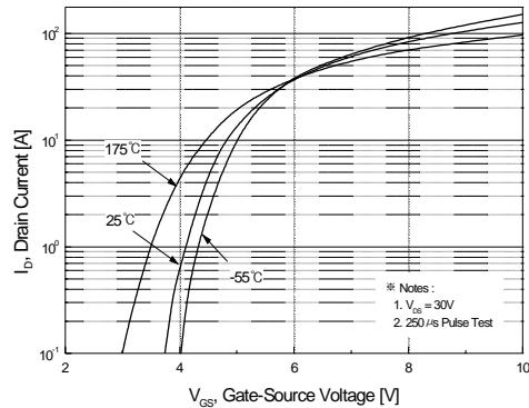
**Figure 2. Transfer Characteristics**
