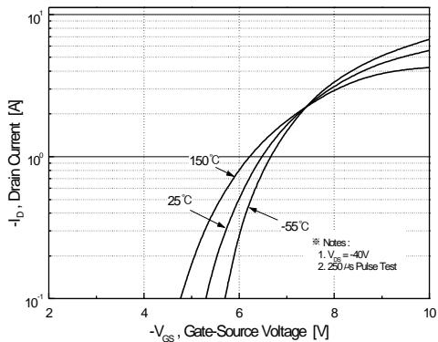
**Figure 2. Transfer Characteristics**
