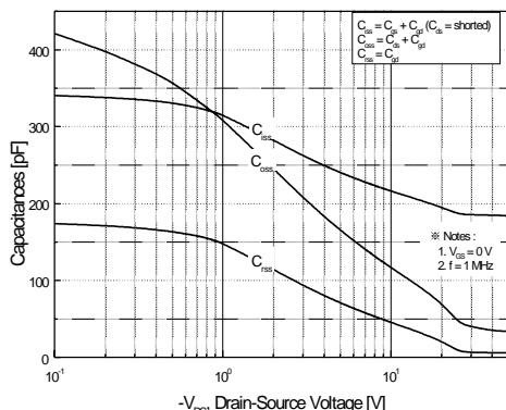
**Figure 5. Capacitance Characteristics**
