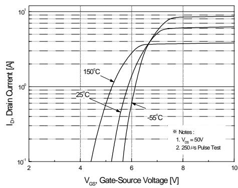
**Figure 2. Transfer Characteristics**
