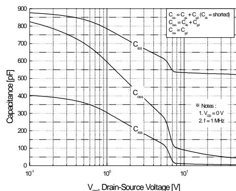
**Figure 5. Capacitance Characteristics**
