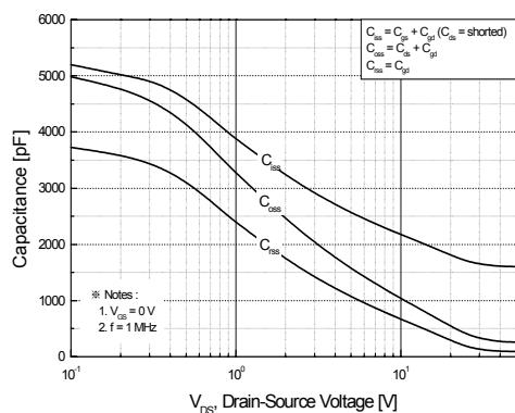
**Figure 5. Capacitance Characteristics**
