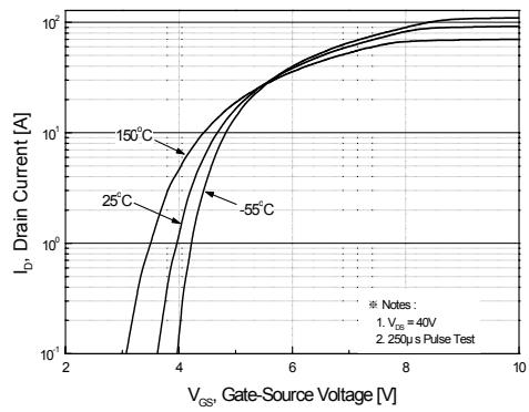
**Figure 2. Transfer Characteristics**
