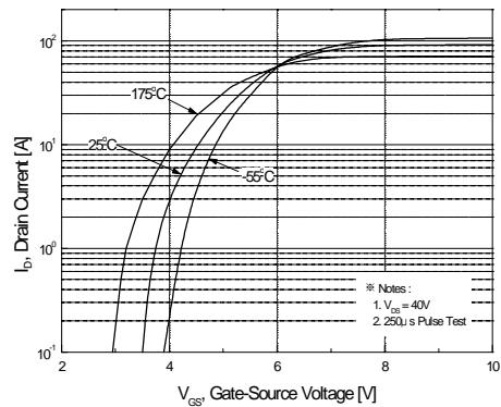
**Figure 2. Transfer Characteristics**
