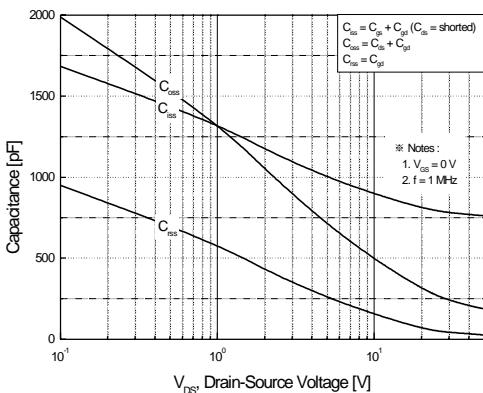
**Figure 5. Capacitance Characteristics**
