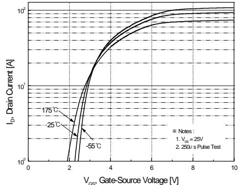
**Figure 2. Transfer Characteristics**
