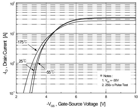
**Figure 2. Transfer Characteristics**
