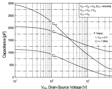
**Figure 5. Capacitance Characteristics**
