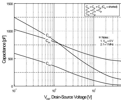
Figure 5. Capacitance Characteristics
