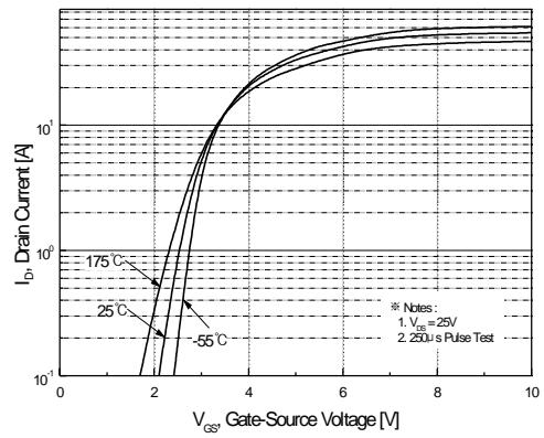
Figure 2. Transfer Characteristics
