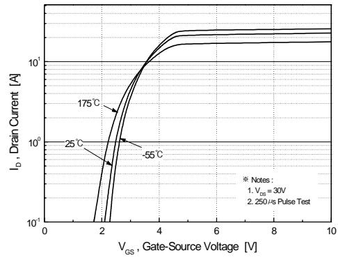
**Figure 2. Transfer Characteristics**
