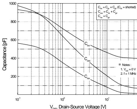
**Figure 5. Capacitance Characteristics**
