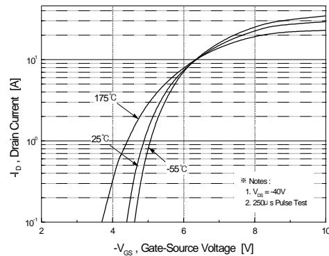
**Figure 2. Transfer Characteristics**
