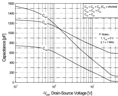
**Figure 5. Capacitance Characteristics**
