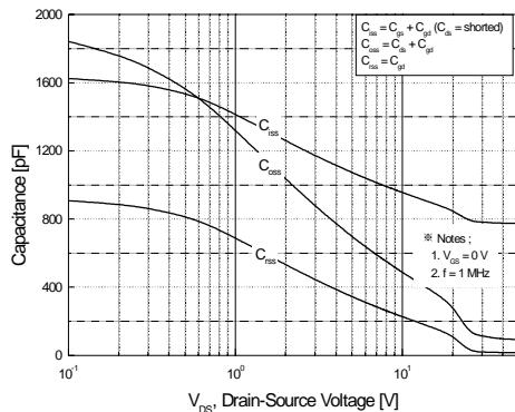
**Figure 5. Capacitance Characteristics**
