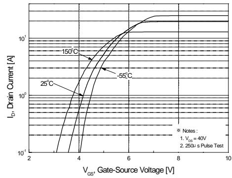
**Figure 2. Transfer Characteristics**
