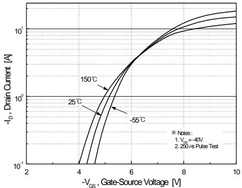
**Figure 2. Transfer Characteristics**
