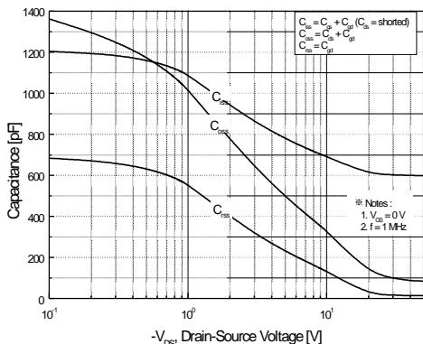
**Figure 5. Capacitance Characteristics**
