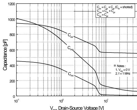
**Figure 5. Capacitance Characteristics**
