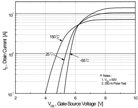
**Figure 2. Transfer Characteristics**
