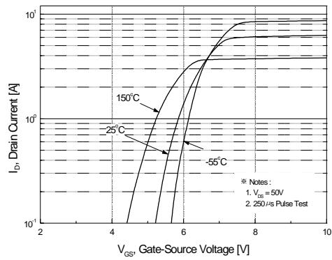
**Figure 2. Transfer Characteristics**
