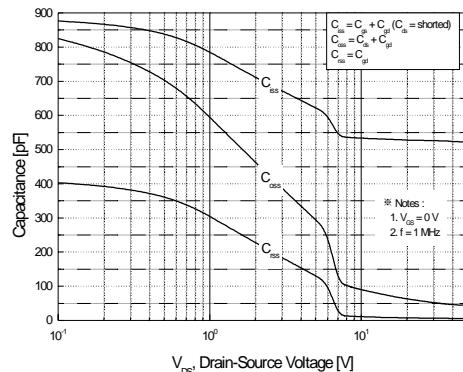
**Figure 5. Capacitance Characteristics**
