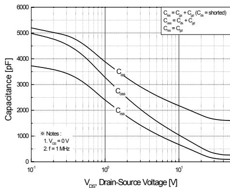
**Figure 5. Capacitance Characteristics**
