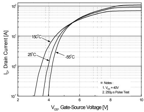
**Figure 2. Transfer Characteristics**
