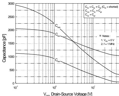
**Figure 5. Capacitance Characteristics**
