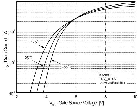
**Figure 2. Transfer Characteristics**
