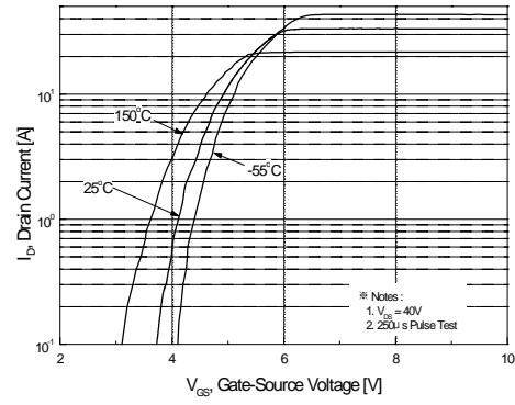
**Figure 2. Transfer Characteristics**
