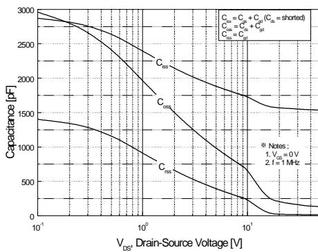
**Figure 5. Capacitance Characteristics**
