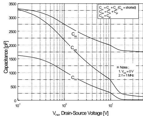
**Figure 5. Capacitance Characteristics**
