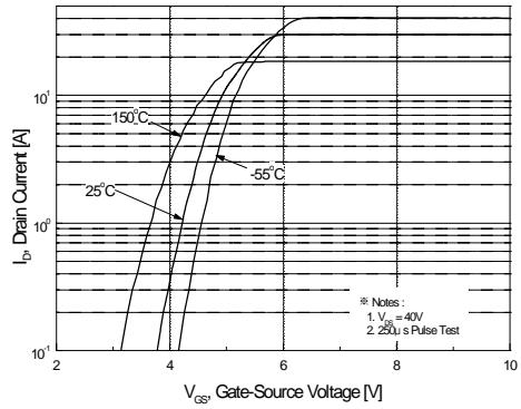
**Figure 2. Transfer Characteristics**
