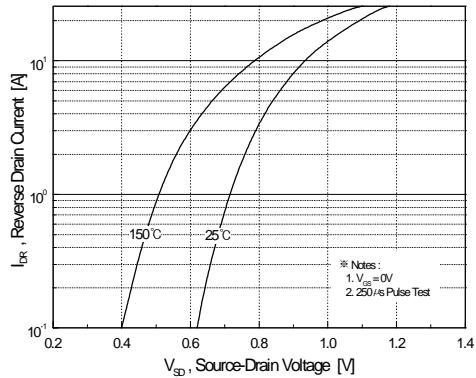
**Figure 4. Body Diode Forward Voltage
