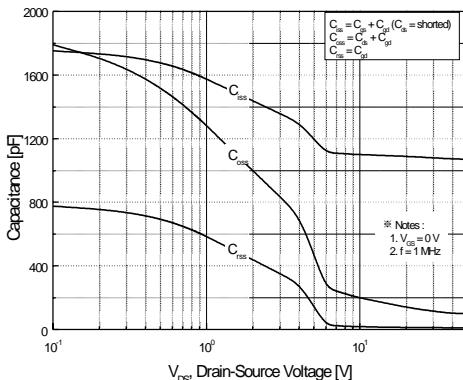
**Figure 5. Capacitance Characteristics**
