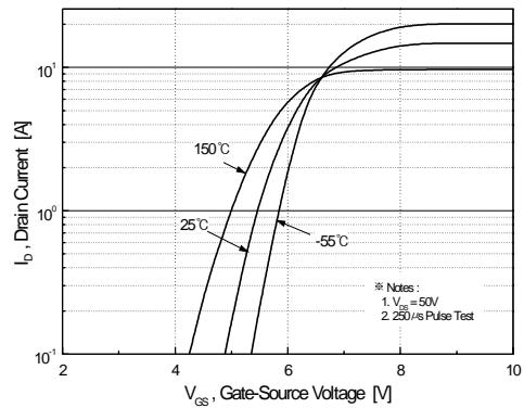
**Figure 2. Transfer Characteristics**
