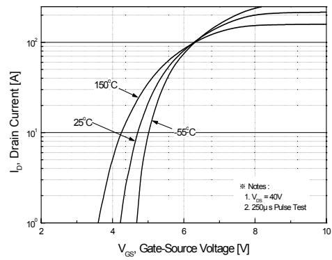
**Figure 2. Transfer Characteristics**
