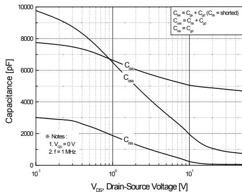
**Figure 5. Capacitance Characteristics**
