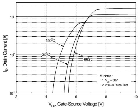
**Figure 2. Transfer Characteristics**
