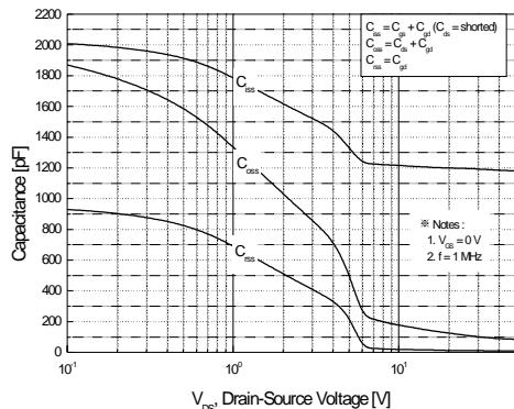
**Figure 5. Capacitance Characteristics**
