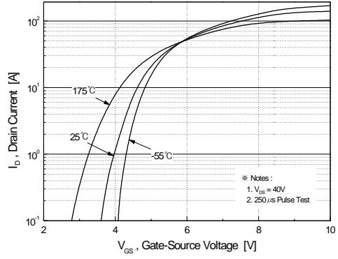
**Figure 2. Transfer Characteristics**
