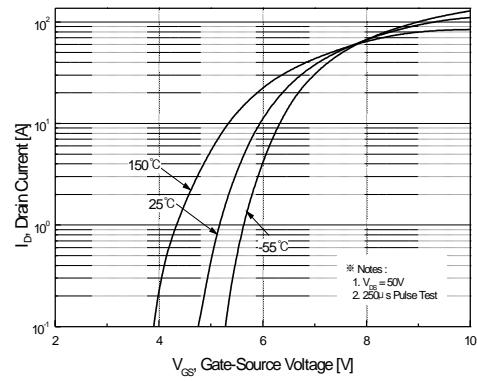
**Figure 2. Transfer Characteristics.**
