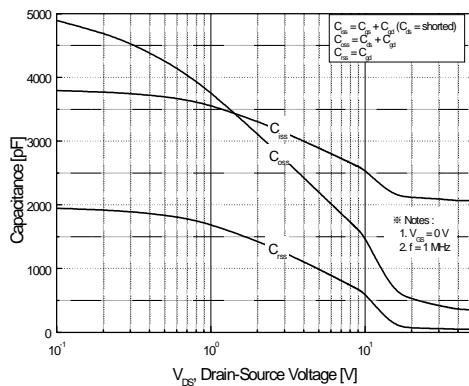
**Figure 5. Capacitance Characteristics.**
