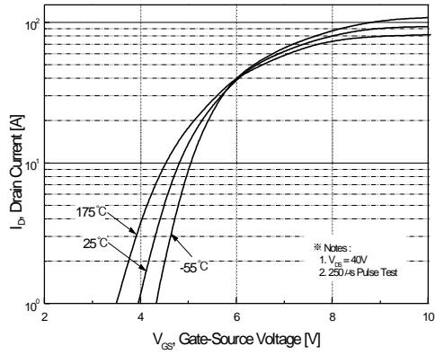
**Figure 2. Transfer Characteristics**
