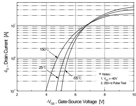
**Figure 2. Transfer Characteristics**
