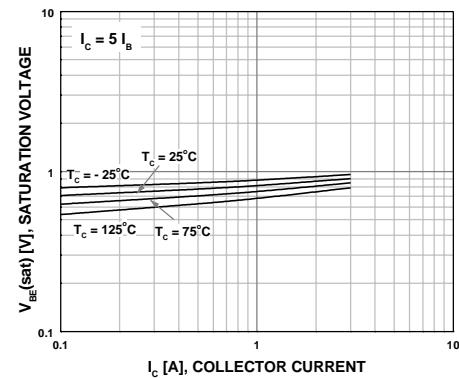
Figure 4. Saturation Voltage
