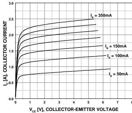
Figure 1. Static Characteristic
