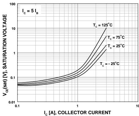
Figure 3. Saturation Voltage
