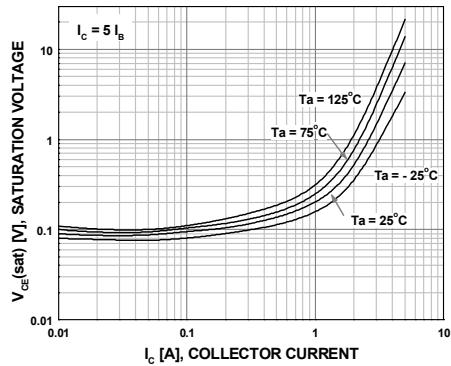
Figure 3. Saturation Voltage
