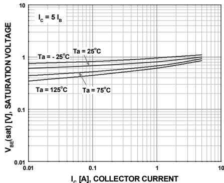
Figure 4. Saturation Voltage
