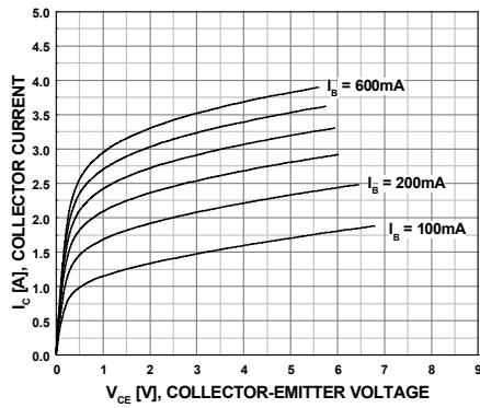
Figure 1. Static Characteristics
