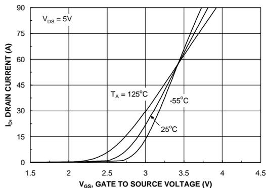
Figure 5. Transfer Characteristics.
