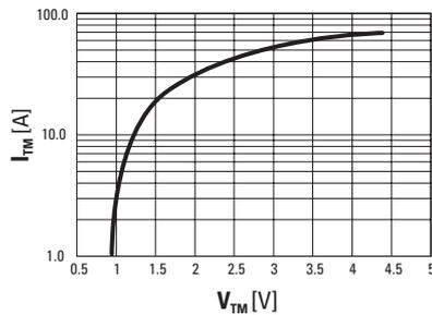
Fig. 3: On-state current versus on-state voltage (instantaneous values)
