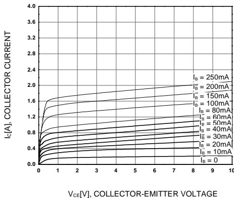
**Figure 1. Static Characteristic**
