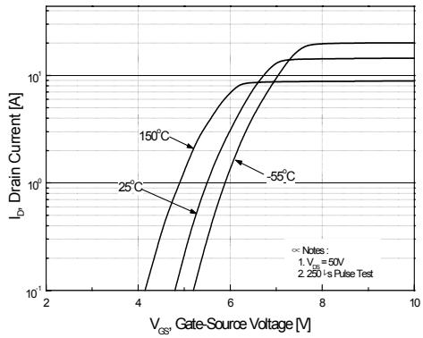
**Figure 2. Transfer Characteristics**
