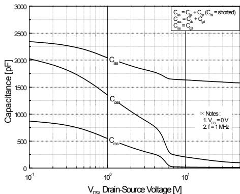
**Figure 5. Capacitance Characteristics**
