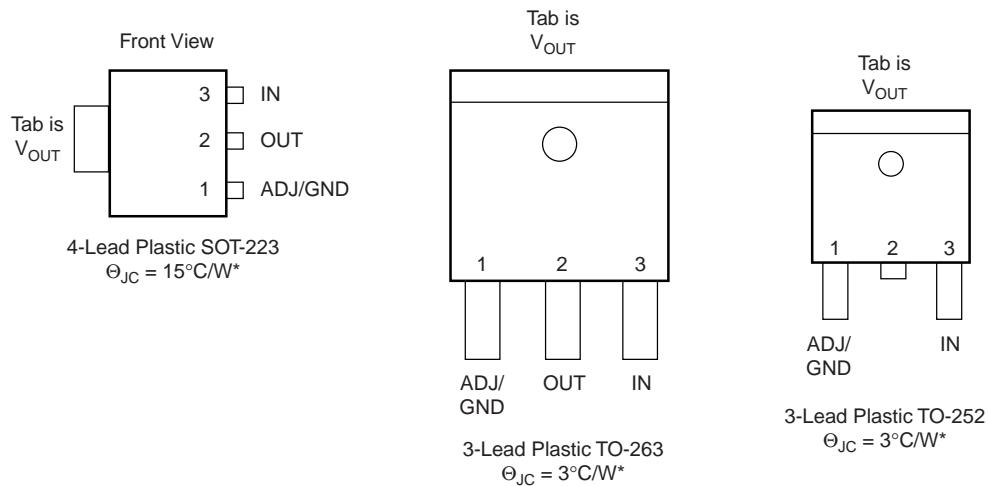
\*With package soldered to 0.5 square inch copper area over backside ground plane or internal power plane,  $\Theta_{JA}$  can vary from 30°C/W to more than 50°C/W. Other mounting techniques may provide better thermal resistance than 30°C/W.
