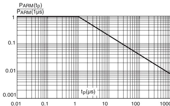
**Figure 5: Non repetitive surge peak forward current versus overload duration (maximum values, per diode) (TO-220AB, TO-247, D<sup>2</sup>PAK)**
