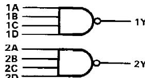
positive logic  $Y = \overline{A} \cdot \overline{B} \cdot \overline{C} \cdot \overline{D}$  or  $Y = \overline{A} + \overline{B} + \overline{C} + \overline{D}$
