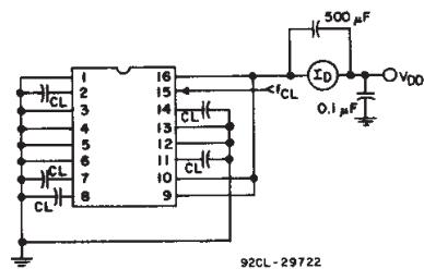
Fig. 13 – Power dissipation test circuit.
