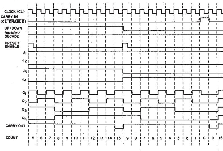
Fig. 10 – Timing diagram-binary mode.
