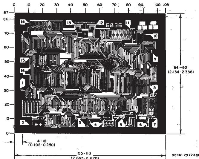
Chip dimensions and pad layout for CD4029B
