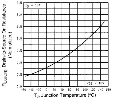
**Fig 4.** Normalized On-Resistance
